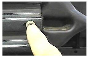
**4.** With a phillips screw driver remove screws from metal bumper ends. Remove end caps and set aside.
