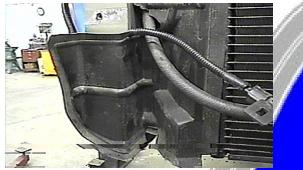
**6.** Remove two push pins on the air dams, both sides and set aside.
