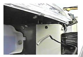
**12.** Drill remaining holes with 13/32 drill bit on the end plates. Use items 3, 4, and 5 according to drawing on last page. Reinstall end caps on metal bumper.
