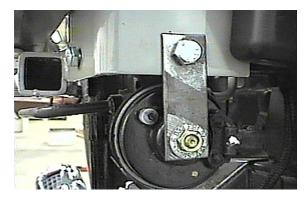
14. Reinstall horn using bracket provided, item9. Be sure to use loctite on all bolts before tightening.
