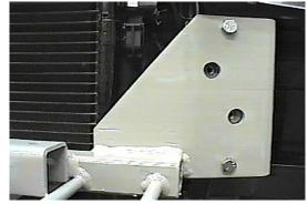
**8.** Hold baseplate in place so that top edge of end plates are flush with top frame webbing. Using the baseplate as a template, drill four holes on the front side of baseplate with the 13/32 drill bit. Insert items 3, 4, and 5, do not tighten.
